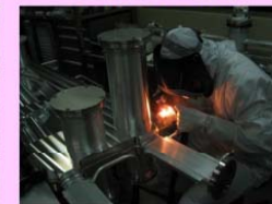
Beam Duct Welding
